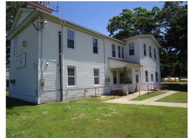
Two rain gardens can be installed on the western side of the building near the entrance to capture, treat, and infiltrate stormwater runoff from the roof. These systems can easily be incorporated into existing landscapes, provide aesthetic value, and create wildlife habitat while managing stormwater runoff. A preliminary soil assessment suggests that more soil testing would be required before determining the soil's suitability for green infrastructure.
